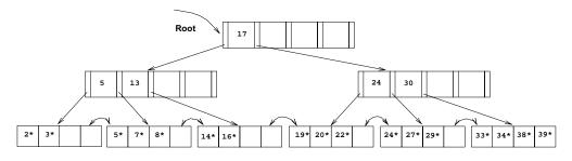
Figure 9.14 B+ Tree after Inserting Entry 8\*
