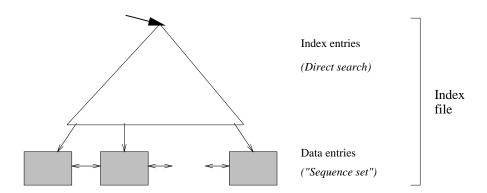
Figure 9.8 Structure of a B+ Tree
