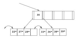
Figure 9.18 Partial B+ Tree during Deletion of Entry 24\*
