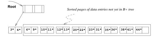
Figure 9.23 Initial Step in B+ Tree Bulk-Loading
