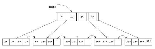
Figure 9.15 B+ Tree after Inserting Entry 8\* Using Redistribution
